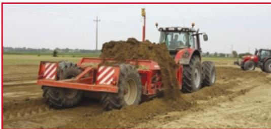
**SCRAPERS IDRAULICI DA MC. 4 A MC. 12 OMOLOGATI A RICHIESTA CON APERTURA FRONTALE DI CARICO A GEOMETRIA VARIABILE IDRAULICA E TELAIO MAGGIORATO. OGNI NOSTRO SCRAPER SI PUÒ AVERE ANCHE IN VERSIONE TRAINANTE PER UTILIZZO IN TANDEM. NELLA FOTO RPS 10 MC.**
